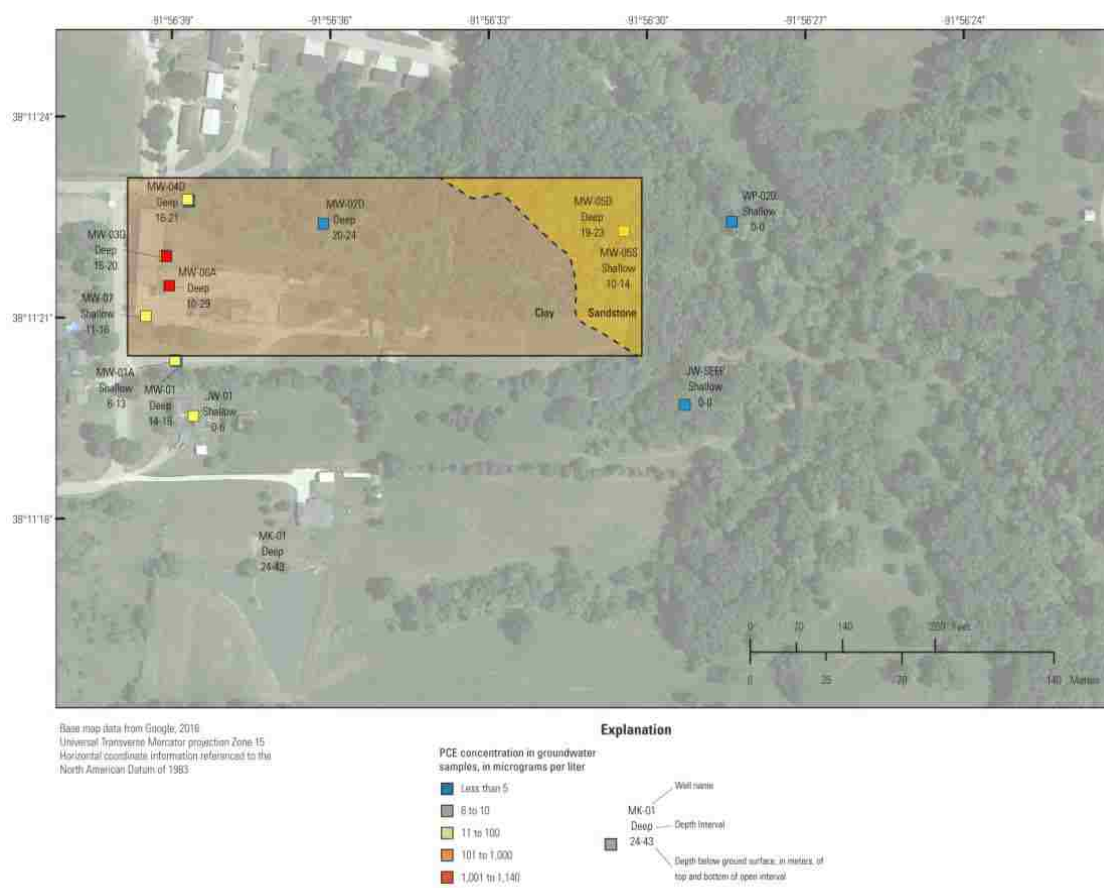
Figure 2. Maximum concentration of tetrachloroethylene (PCE) and construction information in groundwater wells and surficial lithology (primarily clay and sandstone).
