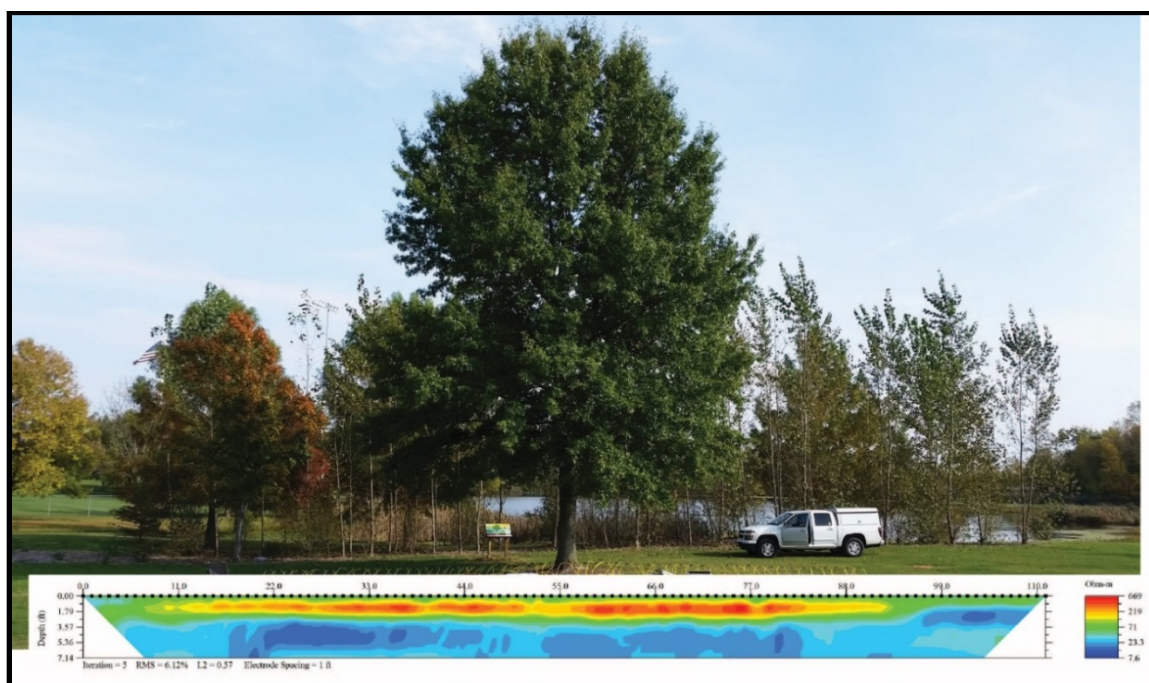
Figure 4.2. Preliminary electrical resistivity data outlining the hypothesized effective root volume (zone of large resistivity) of a large oak tree at Schuman Park in Rolla, MO.
